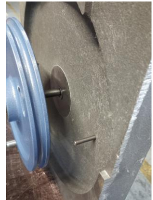
Grooved dowel pins as protection against jumping off and tension pulley with shim washer
