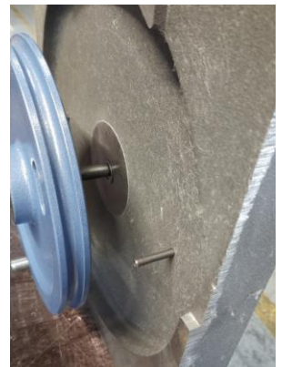
Grooved dowel pins as jump-off protection and tension pulley with shim
