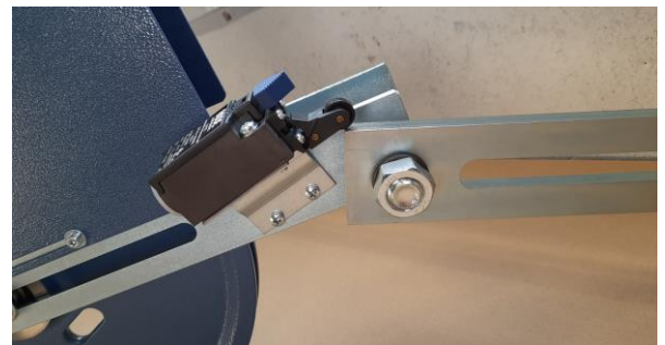
Picture 3: Tension weight is lowered by the elongated GB rope and actuate the slack rope switch
